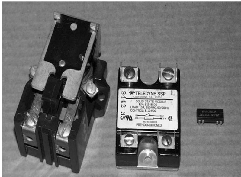
Figure 8.60 Photo of an EM, solid-state, and reed relay.
