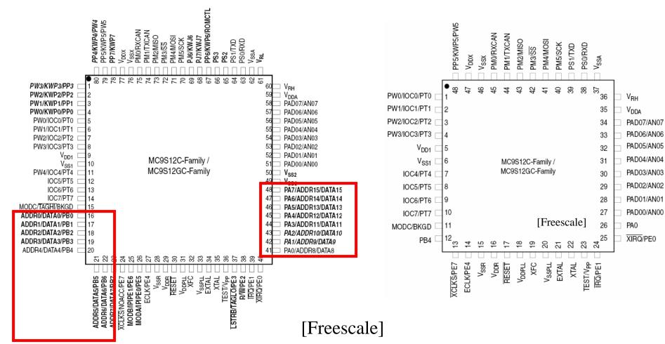
Signals shown in **Bold** are not available on the 52- or 48-pin package Signals shown in **Bold Italic** are available in the 52-pin, but not the 48-pin package
