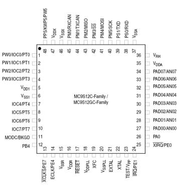
Figure 1-9. Pin Assignments in 48-Pin LQFP
