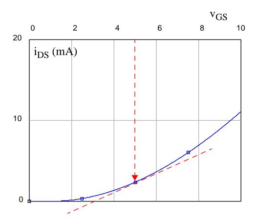
$$g_m = \frac{\partial i_D}{\partial v_{GS}} \bigg|_{v_{GS} = V_{GS}}$$
