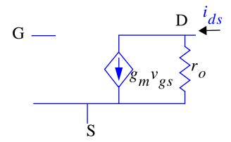
• r<sub>o</sub> is the drain-source voltage change with change in i<sub>ds</sub> due to channel length modulation.
