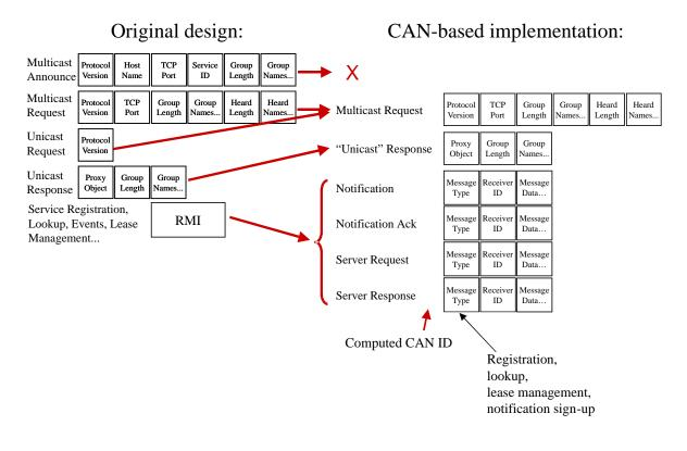
Figure 8: Original Jini modified to work on CAN
