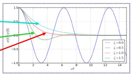
Time dependence of the system behavior on the value of the damping ratio ζ, for undamped (blue), under-damped (green), critically damped (red), and over-damped (cyan) cases, for zero-velocity initial condition.
