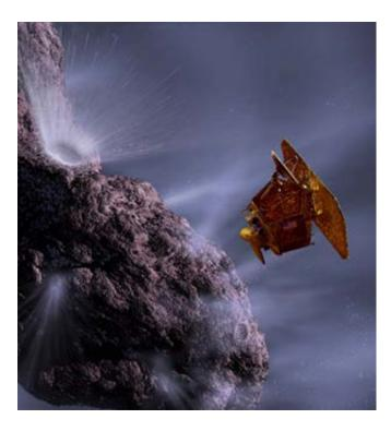
http://apod.nasa.gov/apod/ image/0505/art1\_deepimpact.jpg Launched in 2005, the spacecraft memorably smashed a copper-jacketed probe into the comet Tempel 1 at 22,800 miles an hour (36,700 kilometers an hour) on July 4 of that year. It then flew through the debris cloud to capture the resultant fireworks, the first close inspection of a comet's interior. (See "Deep Impact' Comet Revealed by NASA Flyby.")
