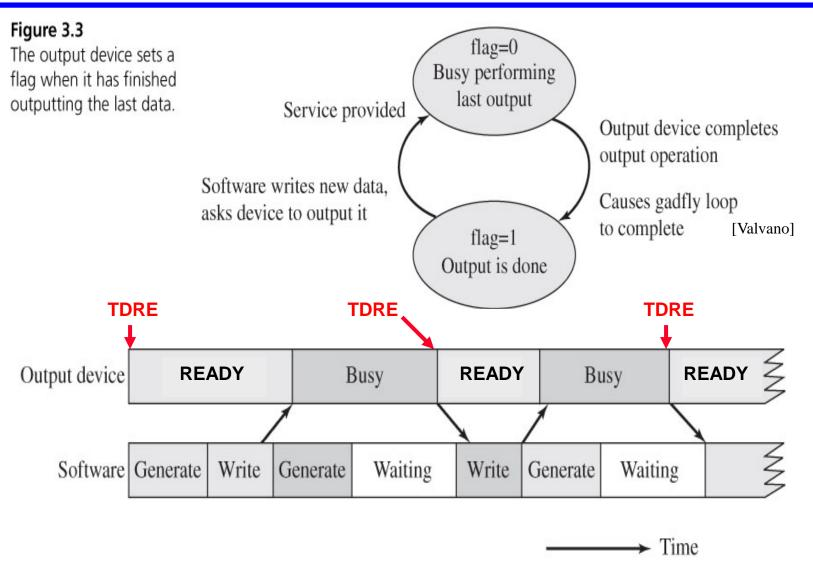
**Figure 3.4**The software must wait for the output device to finish the previous operation.
