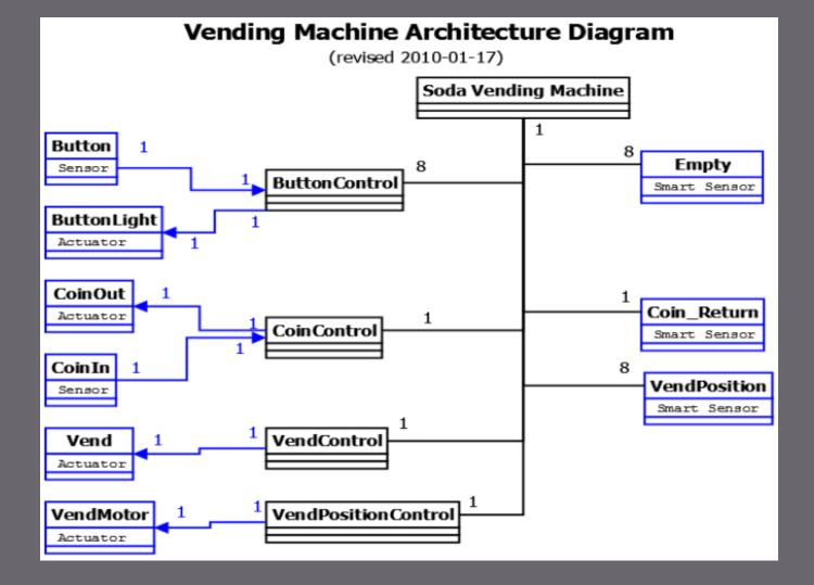
Black line = "is comprised of" Blue line = "analog connection" Numbers are replication counts Black box = SW function Blue box = I/O hardware
