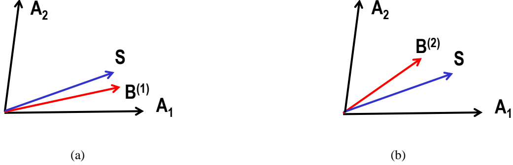
Figure 2-10. A 2-D example of using S-OMP to select the correct basis vector from two choices.
