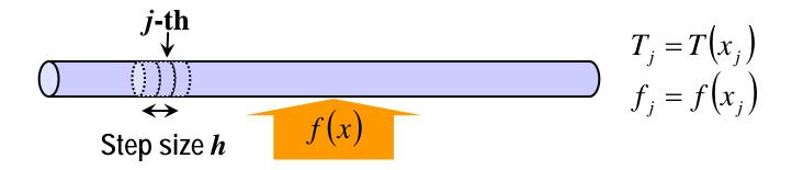
$$T(x=0,t) = T(x=1,t) = 0 \qquad -\kappa \cdot T_{xx}(x) = f(x) \qquad T_{xx}(x_j) = \frac{T_{j+1} + T_{j-1} - 2T_j}{h^2}$$
