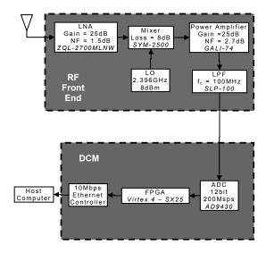
Fig. 3. Data path in the SCM, All parts are from Minicircuits except the ADC and FPGA which are from Analog Devices and Xilinx respectively.
