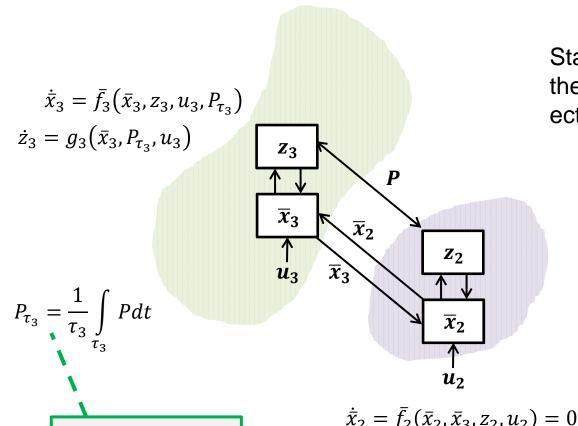
Stabilize interaction variable of the generators module using ectropy
