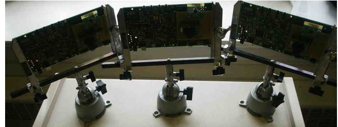
Figure 1 – Three of the prototype VSN nodes. These nodes form a multi-hop wireless mesh network implementing the CDPM policies investigated in this work and the object tracking driver application as described in Section 2.
