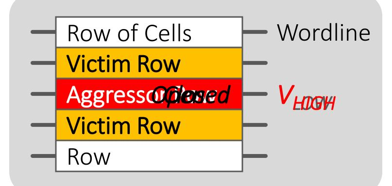
Repeatedly opening and closing a row induces **disturbance errors** in adjacent rows in **most real DRAM chips** [Kim+ ISCA 2014] 36
