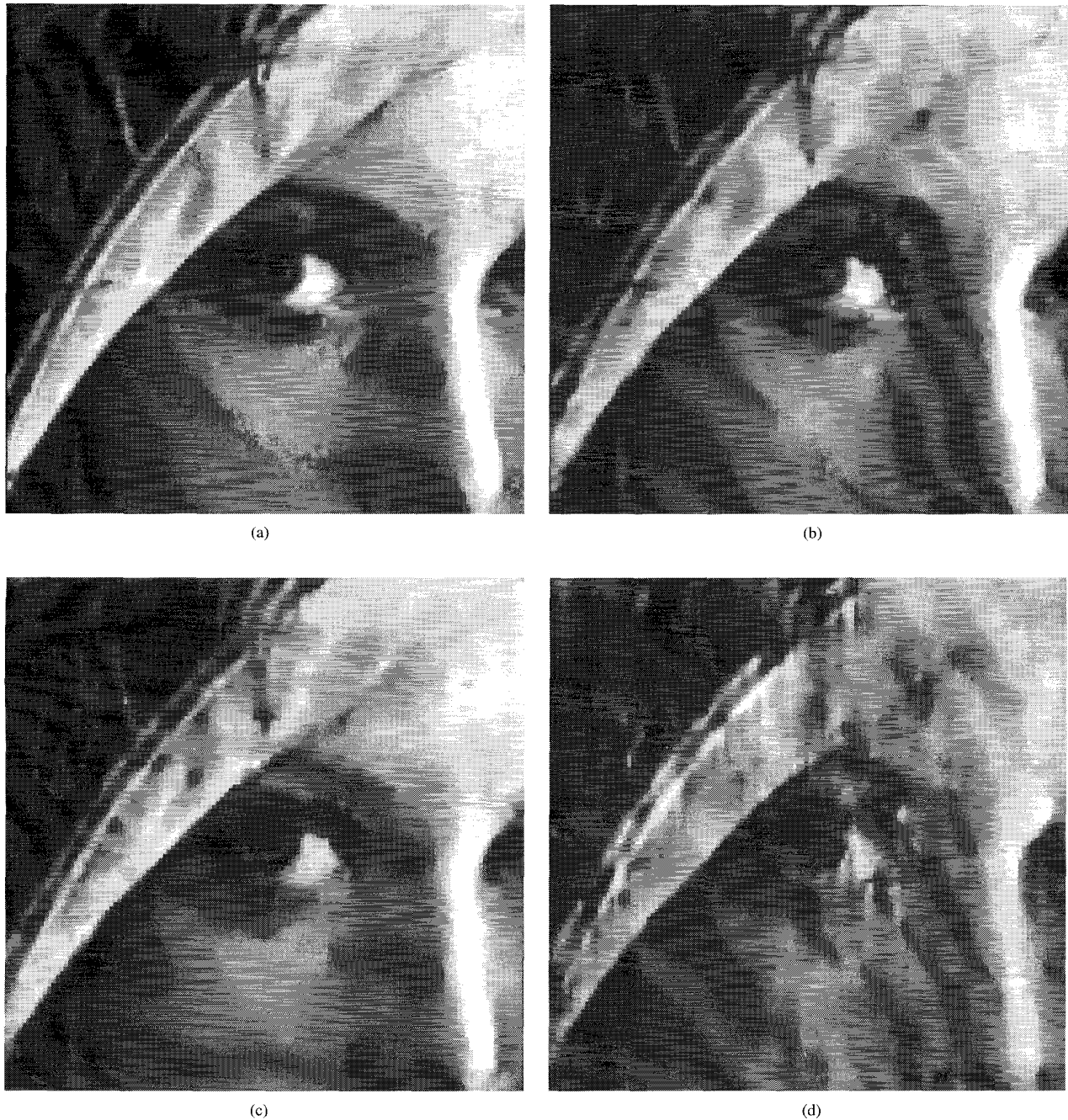
Fig. 5. (a) Original 128 \times 128 Lenna. (b)–(d) Comparison of reconstructed Lenna after compression to 0.375 b/pixel using: (b) NCP-VQ with optimal ML parameters from Table I; (c) NCP-VQ with approximated parameters from Table I; (d) third-order Markov mesh (causal prediction) with optimal parameters from Table I.
