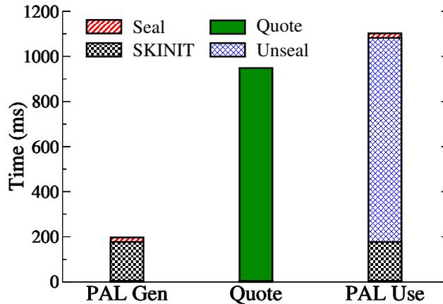
Figure 3.6: Breakdown of overheads that will be incurred by generic applications implemented with Flicker. Measurements were taken using an HP dc5750 containing an AMD processor and a Broadcom TPM. PAL Gen represents the overhead for an application that generates data and seals it for later use. PAL Use unseals previous state, modifies it, and reseals it.
