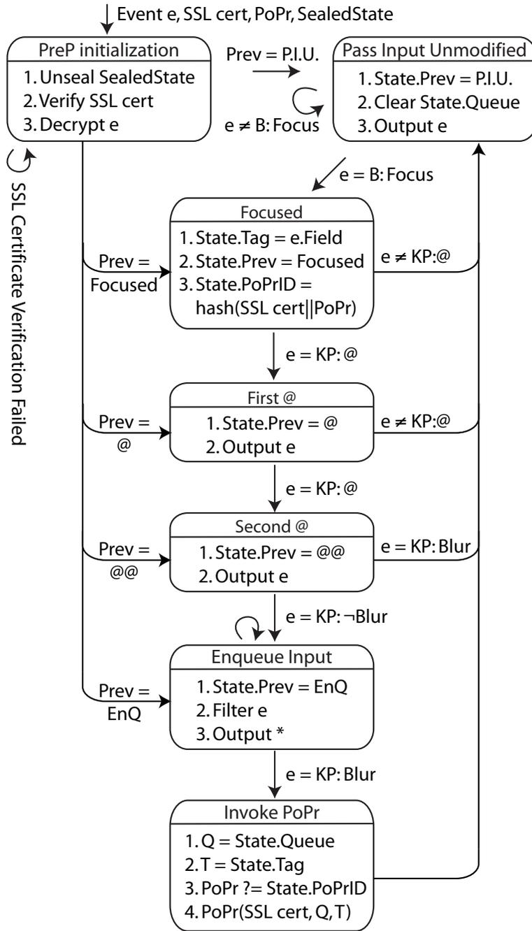
Figure 4.3: States of the PreP. KP = keypress or mouse click. B:Focus = browser GUI *focus* event. Blur indicates action taken in response to events on the encrypted input channel that cause a GUI *blur* event (e.g., Tab, Shift+Tab, Enter, or mouse click).
