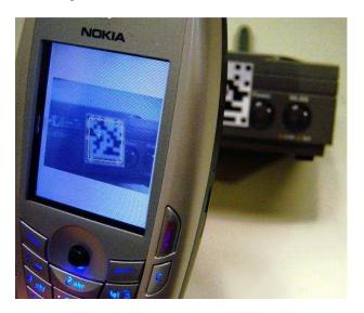
Figure 3. Phone running SiB scanning a barcode on an 802.11 access point.
