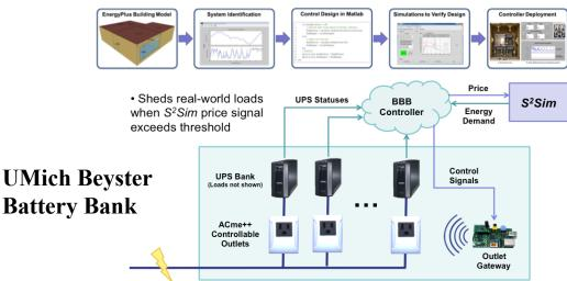
Pricing feedback from S<sup>2</sup>Sim based on consumption, affects appliance rescheduling, battery charge/discharge periods, matching solar energy with demand
