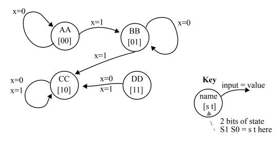
The machine above has four states AA BB CC DD, represented by 2 bits of state (2 flip flops) whose values appear in brackets (e.g., [10] represents state CC) in each state bubble. This machine has just 1 input x. We are ignoring any outputs for this machine.
