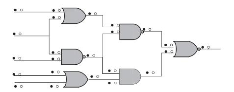
Use deductive fault simulation to determine all of the faults found by the test 0111 in the circuit below. Show the list of visible faults for each node. For each node beyond the inputs, show the equations used to find the list. What faults are finally detected at the output?
