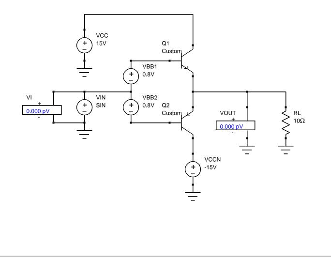
• Input and output are now overlapping, with no cross-over distortion
