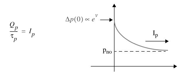
• SPICE models this in terms of an average transit time, the average time a hole stays in the n region of the diode (or: an electron stays in the p region)
