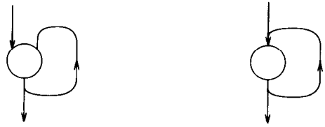
Figure 7. Problems with cyclic graphs. The graph on the left will deadlock; the one on the right will never finish.
