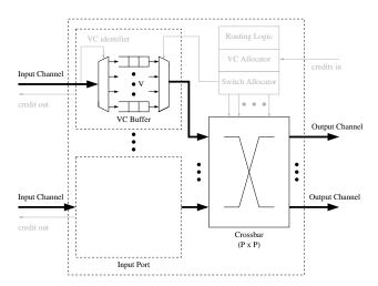
Figure 2. Virtual-Channel Router
