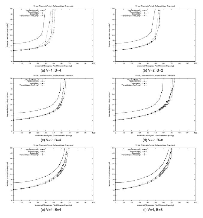
Figure 9. Latency versus throughput for a number of different VC and switch allocation implementations (5-flit packets). For each graph,  $\forall$  is the number of virtual-channels per input port and  $\exists$  is the number of buffers per virtual-channel.
