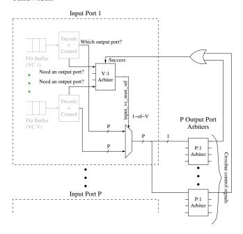
Figure 4. Switch Allocation Logic
