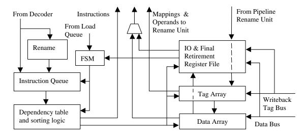
Figure 3: The trace buffer block diagram
