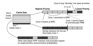
Figure 9: Example organization of the In-Cache Estimation Monitors (ICEmon) for two cores sharing an eight-set, eightway cache.
