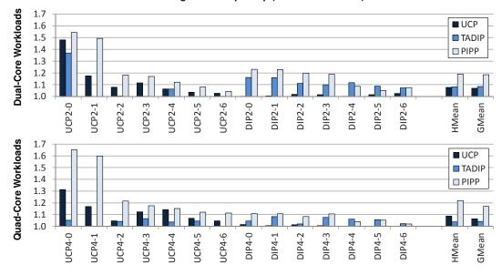
Figure 4: Performance as measured by the weighted speedups of IPC for UCP, TADIP and PIPP normalized to an LRU-managed cache for dual-core and quad-core workloads.
