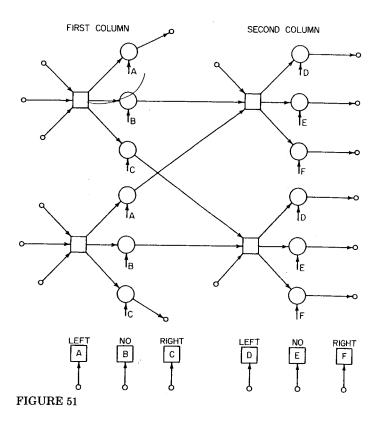
and left shifts. This assumes that only two bits of network are contained on a module.
