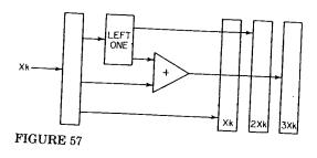
When these multiples of the multiplicand Xk are available, a sequence of four identical steps is taken utilizing the two halves of the multiplication. Each of the four steps accomplishes the multiplication of six bits in each half. This is diagrammed in Figure 58, showing three "carry-save" layers of network followed by a holding register.
