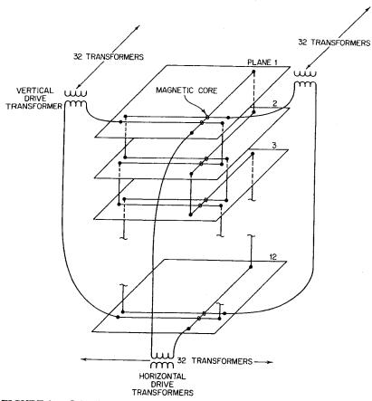
FIGURE 31 Drive line connections.
