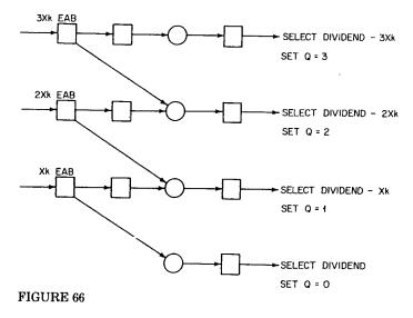
This logic is a direct result of the relationship of end-around-borrow to the relative sizes of the partial dividends and the particular subtractor. There will be an EAB only if the applicable divisor multiple is greater than the dividend.
