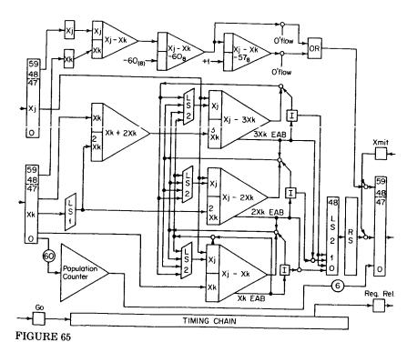
and its second and third multiple, a design condition rather similar to the Multiply Unit. Because the operands are initially forced positive, the dividend is positive and the divisor is negative in preparation for the subtraction.
