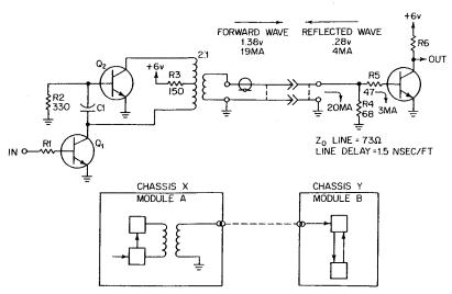
FIGURE 21 Coaxial cable driver.
