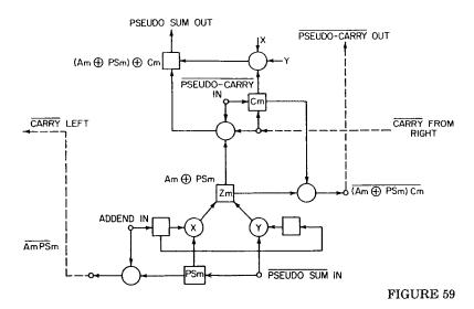
sum is formed using the "inputs" of Zn and Cn to obtain the NOT or complement of each. The purpose is both total hardware and time through the network, the second being most important. If, for example, an additional term were included for  $\overline{Zn}$ , this additional inverter time would be added to the network. The maximum number of inverters through the network is five.
