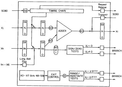
FIGURE 48 Long add unit-block diagram.
