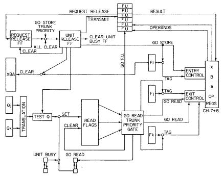
FIGURE 80 Request release block diagram.
