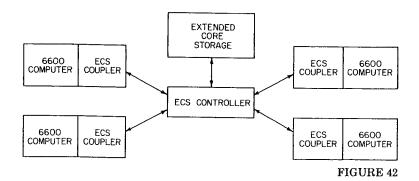
The ECS Coupler can be thought of as a functional unit of the 6600 CPU. However, no attempt is made to allow concurrent operation between it and other functions. In fact, any continuous transfer requires complete control over Central Storage. The CPU provides three items of data to perform the transfer.
