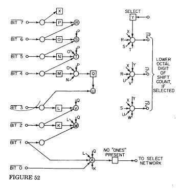
The first test is accomplished by a simple test of each bit of eight compared with the bits more significant in the group. A three-bit number is formed directly from the logic, and a zero test of all bits is also formed.
