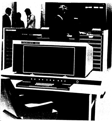
Operator console with keyboard and display.
