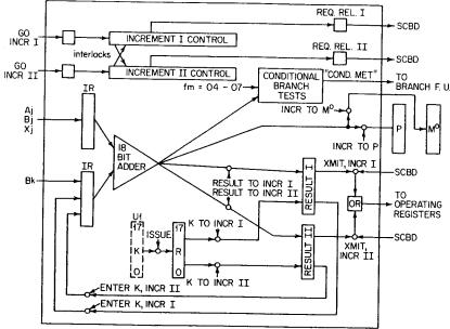
FIGURE 69 Increment functional units-block diagram.
