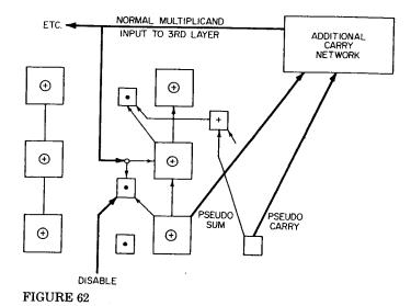
brought into the input normally used by the multiplicand for the bottom layer. Similarly, the pseudo-carry from the "upper" half partial product is brought into the middle layer. See Figure 63. The carry from the lower 24 bits of product is introduced into the long carry network as shown.
