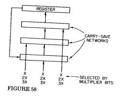
Each carry-save layer forms the sum of the partial product and the multiplicand "multiple" selected by two bits of the multiplier. The result of this sum is passed on to the next layer, shifted to the right two bit positions. The value placed in the holding register at the end of each step is the partial
