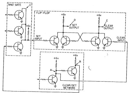
FIGURE 18 Basic flip-flop with clear/set input.
