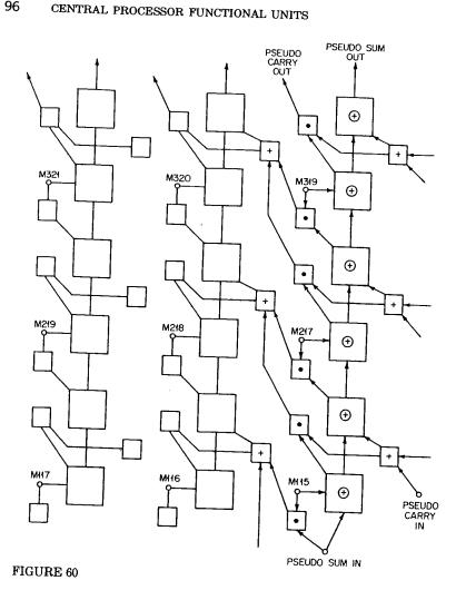
multiplicand terms are defined as M117, M217, and M317, showing the independence of each layer in terms of multiple selection but retaining the bit identification. These three are all bit 17 of the selected multiple.
