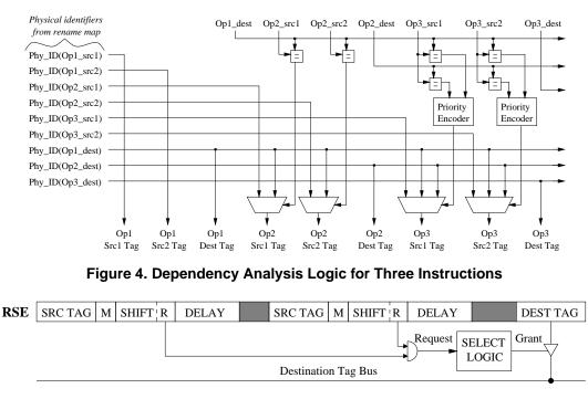
Figure 5. Scheduling Logic for One Reservation Station Entry
