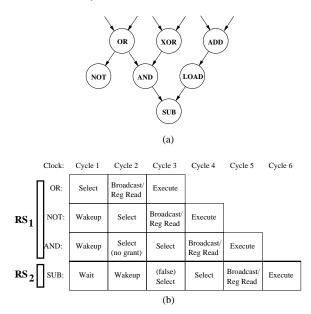
Figure 11. Example of Speculative Wakeup
