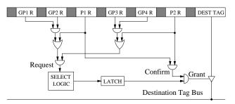
Figure 10. Speculative Wakeup Logic
