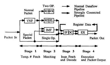
Figure 9 Pipeline Organization of the EMC-R.
