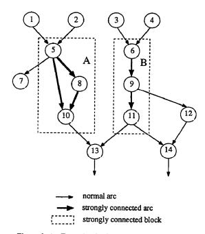
Figure 1 An Example of a Strongly Connected Block.
