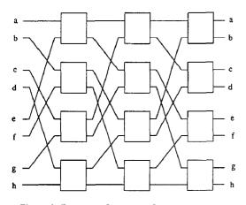
Figure 2 Processor Connected Omega Network.
