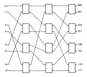
Figure 5. An 8 x 8 delta network to allow identity permutation.
