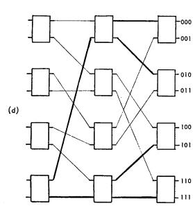
Figure 4. Construction of an 8 x 8 delta network.
