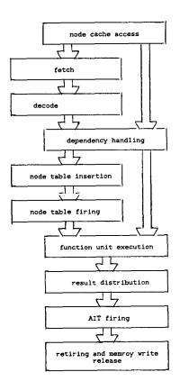
Figure 3. Pipelined View of HPSm
