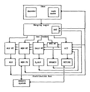
Figure 2. HPSm Data Path
