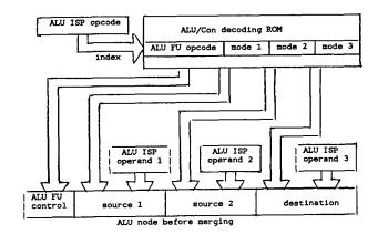
Figure 4. ALU Operation Decoding
