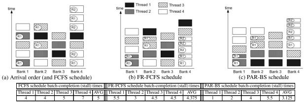
Figure 3. A simplified abstraction of scheduling within a batch containing requests from 4 threads. Rectangles represent marked requests from different threads; bottom-most requests are the oldest requests for the bank. Those requests that affect or result in row-hits are marked with the row number they access; if two requests to the same row are serviced consecutively, the second request is a row-hit with smaller access latency. The first request to each bank is assumed to be a row-conflict
