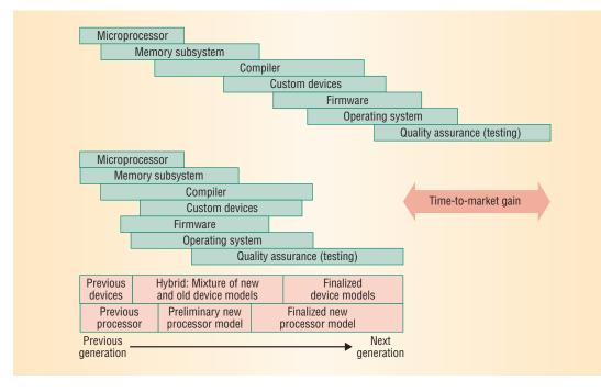
Figure 3. Task dependencies for developing a highend digital system (top) are relaxed in full system simulation (middle), reducing time to market.
