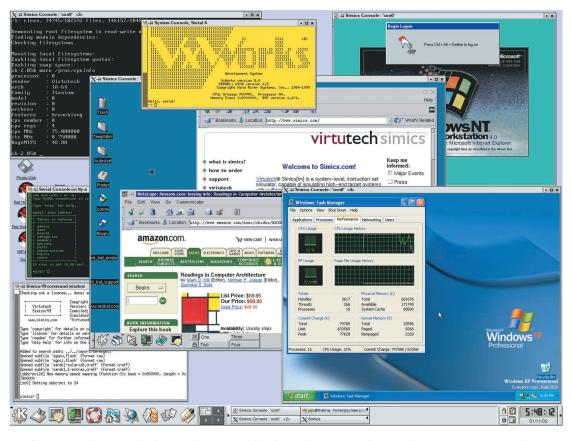
Figure 1. Simics simulation of target systems based on several processor architectures. Each simulated system can run unmodified operating systems and applications.
