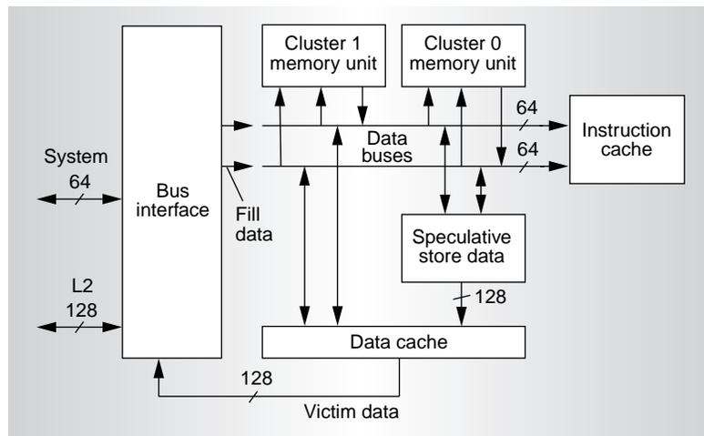
Figure 7. The 21264's internal memory system data paths.
