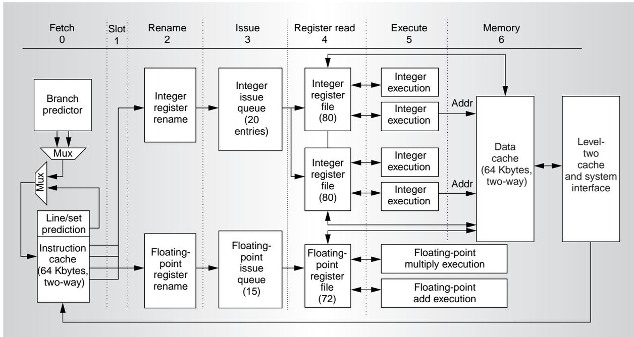
Figure 2. Stages of the Alpha 21264 instruction pipeline.
