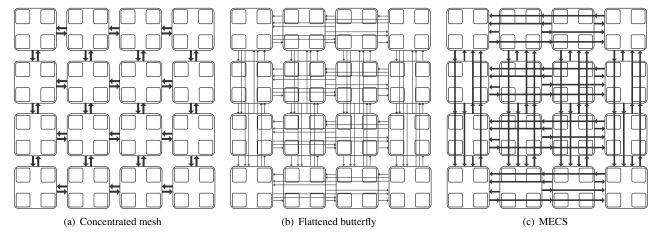
Figure 1. Concentrated Mesh, Flattened Butterfly and MECS topologies for a 64-terminal network.
