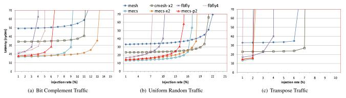
Figure 5. Load-latency graphs for 256-node mesh, CMesh, flattened butterfly and MECS topologies.
