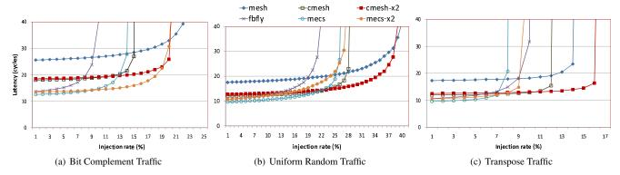
Figure 4. Load-latency graphs for 64-node mesh, CMesh, flattened butterfly and MECS topologies.
