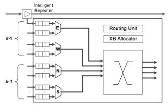
Figure 2. MECS router microarchitecture.
