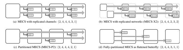
Figure 3. MECS variants for cost-performance trade-off. Only one dimension is shown for simplicity.
