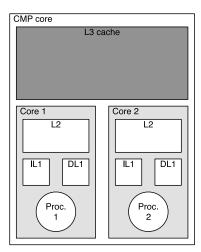
Figure 9: Multicore architecture simulated
