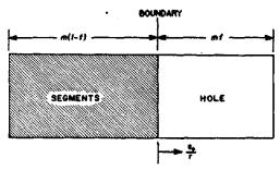
FIG. 9. Configuration of memory after compaction
