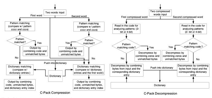
Fig. 2. C-Pack (a) compression and (b) decompression.
