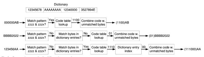
Fig. 3. Compression examples for different input words.
