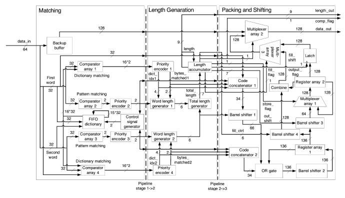
Fig. 6. Compressor architecture.
