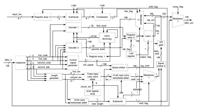
Fig. 7. Decompressor architecture.
