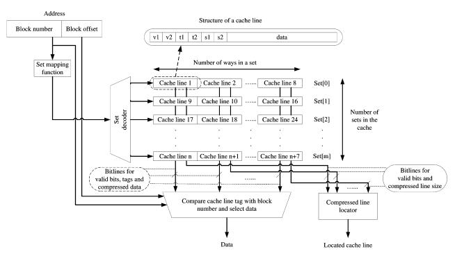
Fig. 4. Structure of a pair-matching based cache.
