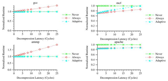
Figure 9. Sensitivity of adaptive compression to decompression latency. *Adaptive* performs the same as the better of *Never* and *Always*, except for mcf.
