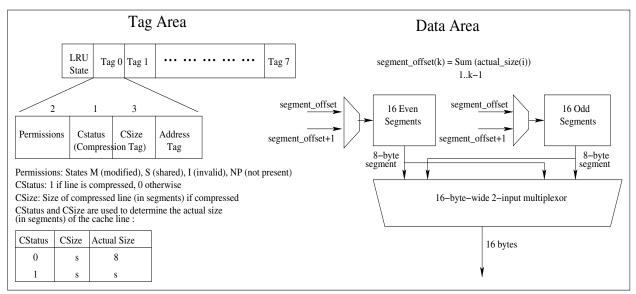
Figure 2. A single set of the decoupled variable-segment cache.
