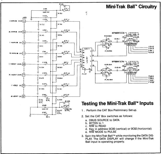
The hardware was implemented according to the original schematic above. Both trackballs were fed into a multiplexer which selects the trackball to monitor. The vertical and horizontal pairs of signals were put into single bit flip flops to hold the direction across a roll. Then, these were fed into incrementing/decrementing counting chips. The 4 bit outputs from these were then sent to the data bus back to the MOS 6502 processor.
