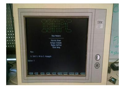
In our original plan, we had endeavored to have a functioning floppy disk drive for demo. This would have enabled us to load in programs from simulated floppy disks. However, the floppy subsystem was far too complex for the amount of time we had available to us. Instead, we developed a keyboard loader system that stored the keystrokes of a BASIC program that we could show off for demo.
