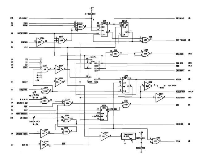
The second section of the motherboard is a complex web of combinational and sequential logic to determine several system signals. These signals handle such jobs as DMA transfers, bus arbitration, NMI, device reset, and I/O check. For this section, we decided to copy the combinational and sequential logic directly from the IBM PC documentation.
