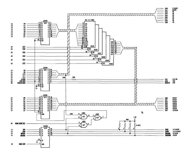
The fifth section of the motherboard contains the ROM. The ROM consists of eight banks, each of which is eight kilobytes, adding up to a total ROM size of 64 kilobytes. The ROM covers addresses 0xF0000 to 0xFFFFF. The first 16 kilobytes are reserved because the original IBM PC had only six banks of memory. The BIOS images we obtained were 64 kilobytes, hence we have instantiated eight banks of memory. These images leave the first sixteen kilobytes free.
