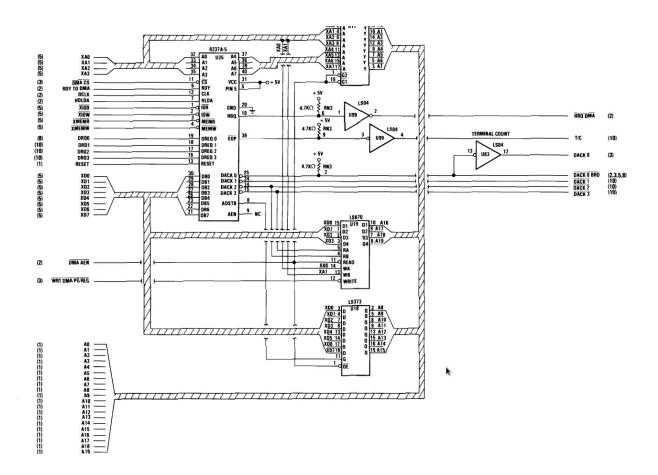
The fourth section of the motherboard consists of the 8237 DMA controller and its associated support chips. The purpose of this module is to perform DMA reads and writes. It includes latches to grab data from I/O devices and send it to memory. Most of the DMA operation takes place within this module.
