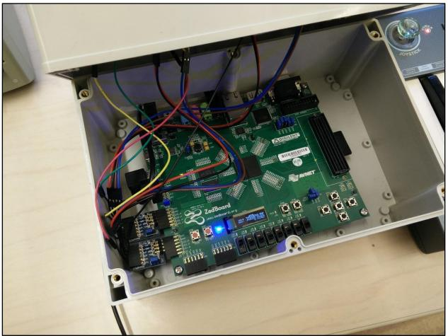
The current status of this project can be seen in the following youtube clip which was taken on the day of the final public demo. The parameter control unit, monophonic scheduler, MIDI over USB interface, processor-logic connection, tone generators, adjustable effects (tremolo and duty cycle), and audio codec were all functional for our public demo.
