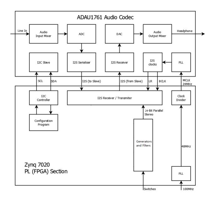
The generated signals from other programmable logic will be passed from the I2S transmitter to the I2S receiver on the codec. Then it will be feed to the DAC on chip and an audio output mixer will output the sound through the speakers connected to the Zedboard.
