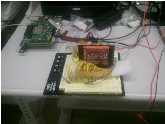
Figure 9. Sega Genesis cartridge breakout board.
