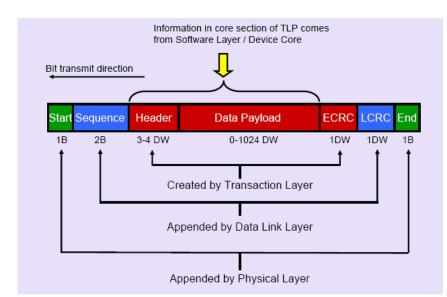
The next important point is packet generation. This is the portion of the specification that will be most valuable in understanding to get a good idea in how the Xilinx blocks work as they do. PCI-E is a layered protocol, consisting
