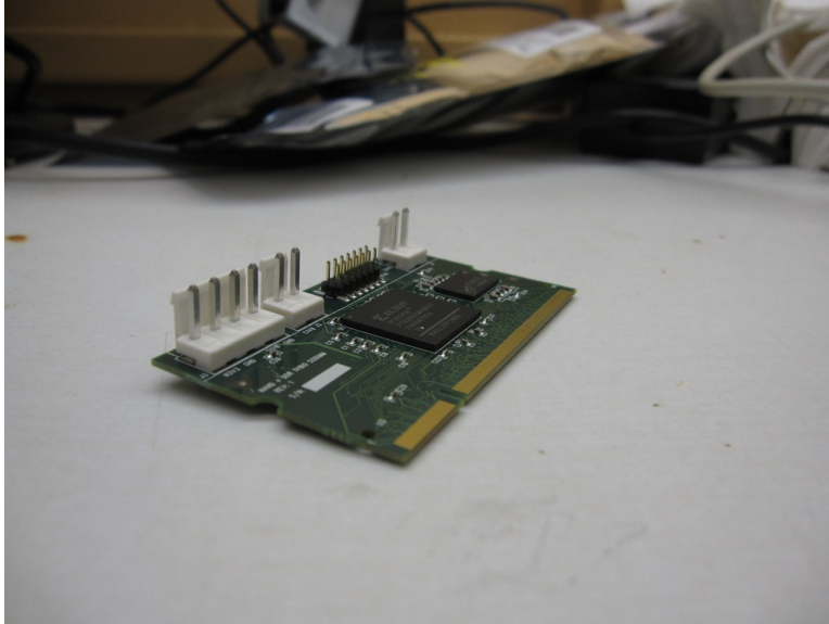
Figure 13: Frontal view of the custom-fabricated SODIMM
