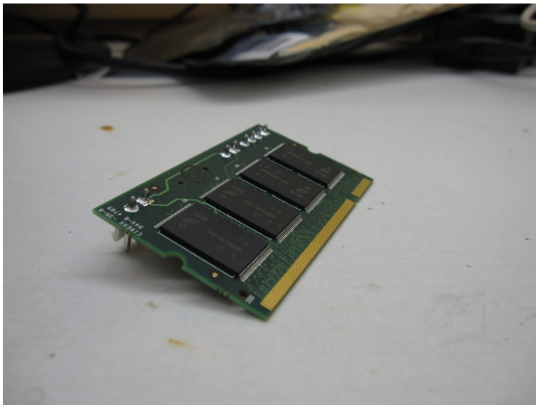
Figure 14: Rear view of the custom-fabricated SODIMM
