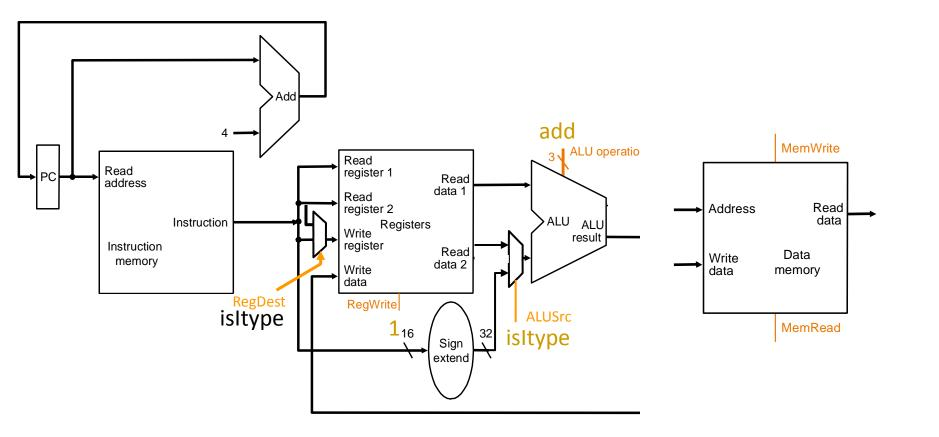
if MEM[PC]==LW rt offset<sub>16</sub> (base) EA = sign-extend(offset) + GPR[base] GPR[rt]  $\leftarrow$  MEM[ translate(EA) ] PC  $\leftarrow$  PC + 4 IF ID EX MEM[WB Combinational state update logic 16
