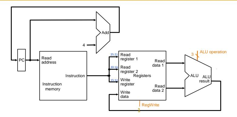
if MEM[PC] == ADD rd rs rt  $GPR[rd] \leftarrow GPR[rs] + GPR[rt]$   $PC \leftarrow PC + 4$ IF ID EX MEM WB Combinational state update logic
