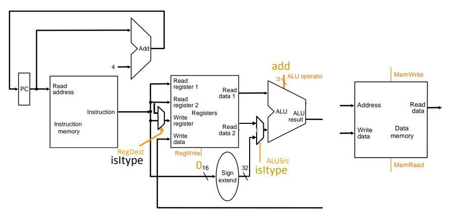
if MEM[PC]==SW rt offset<sub>16</sub> (base) EA = sign-extend(offset) + GPR[base] MEM[ translate(EA) ]  $\leftarrow$  GPR[rt] PC  $\leftarrow$  PC + 4 IF ID EX MEM WB Combinational state update logic 18
