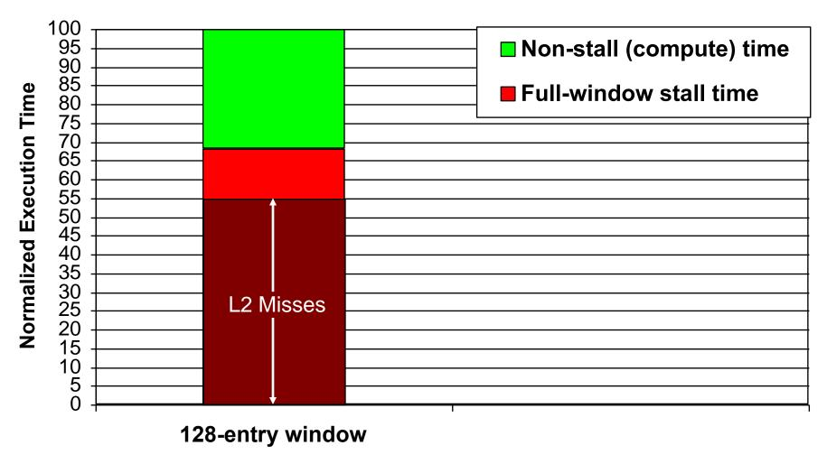
512KB L2 cache, 500-cycle DRAM latency, aggressive stream-based prefetcher Data averaged over 147 memory-intensive benchmarks on a high-end x86 processor model
