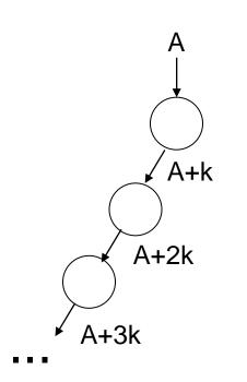
A **traversal address load** loads the pointer to next node:
