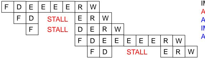
$\begin{array}{cccc} \text{IMUL} & \text{R3} \leftarrow \text{R1}, \text{R2} \\ \text{ADD} & \text{R3} \leftarrow \text{R3}, \text{R1} \\ \text{ADD} & \text{R1} \leftarrow \text{R6}, \text{R7} \\ \text{IMUL} & \text{R5} \leftarrow \text{R6}, \text{R8} \\ \text{ADD} & \text{R7} \leftarrow \text{R3}, \text{R5} \end{array}$
