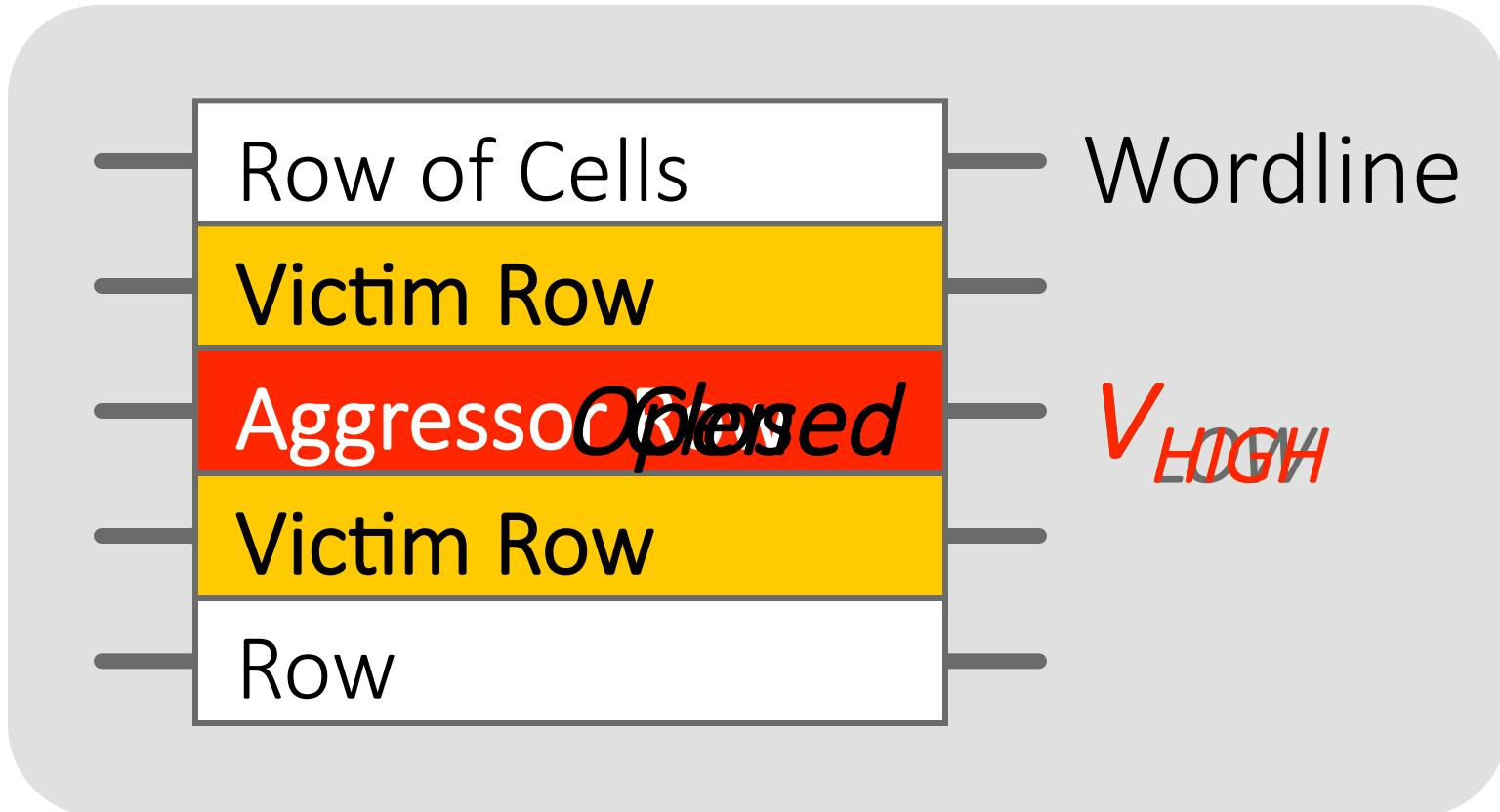
Repeatedly opening and closing a row enough times within a refresh interval induces **disturbance errors** in adjacent rows in **most real DRAM chips you can buy today**
